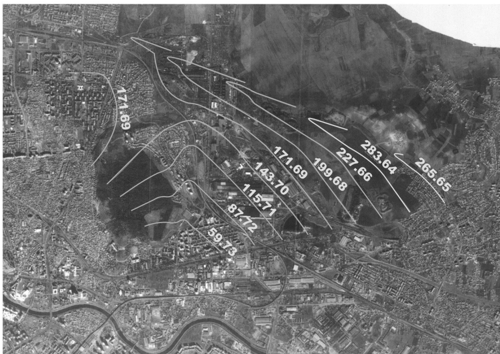
Figure 9. Image of technogenic dust and toxic substances dispersion in the atmosphere - \text{SiO}_2 ( \text{mg}/\text{dm}^3 )
