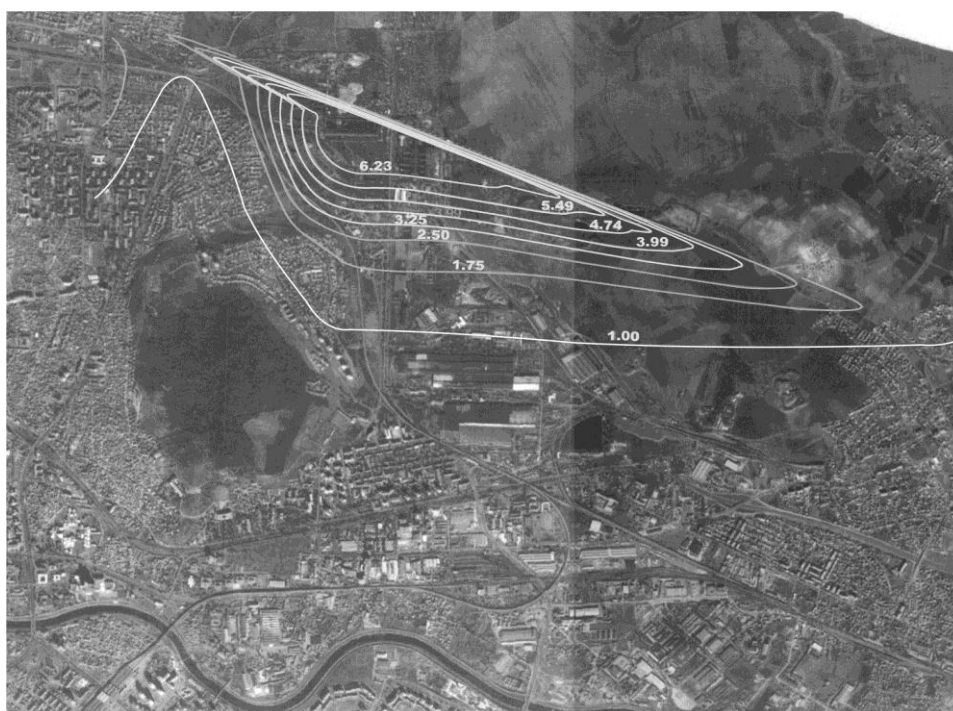
Figure 8. Image of technogenic dust and toxic substances dispersion in the atmosphere - \text{MnO}_2 ( \text{mg}/\text{dm}^3 )
