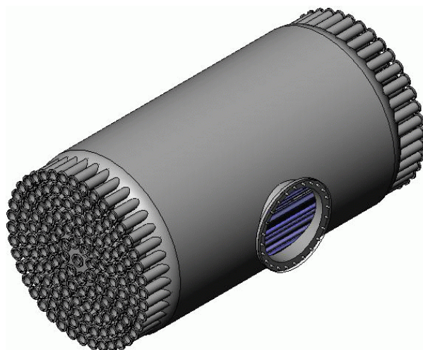
Figure 4. High capacity multi-lamp cylindrical UV reactor with neutral radiation geometry [1,10]; for capacities \geq 1 \text{ m}^3/\text{s}
