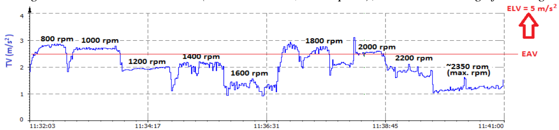
Figure 10. Time history ( a_{hv} in time domain) for HAV on AGT's steering wheel – service condition 4 (vehicle speed 0 km/h, no load, and partial to full throttle).
