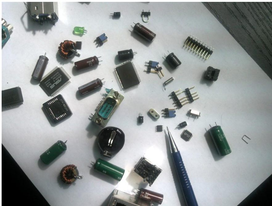
Figure 4. Some disassembled electronic components detached under their own weight
