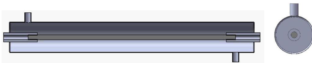
Figure 1. Cylindrical UV reactor with one centrally positioned UV lamp, with negative radiation geometry [1,9]; longitudinal and perpendicular cross section
